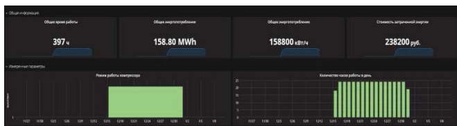
Fig. 4. Appearance of the energy specialist's workstation interface for displaying statistics of the compressor operation using the dark background of the screen form
